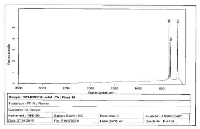
Figure 1. Raman spectrum of Dipotassium hexachloroplatinate
