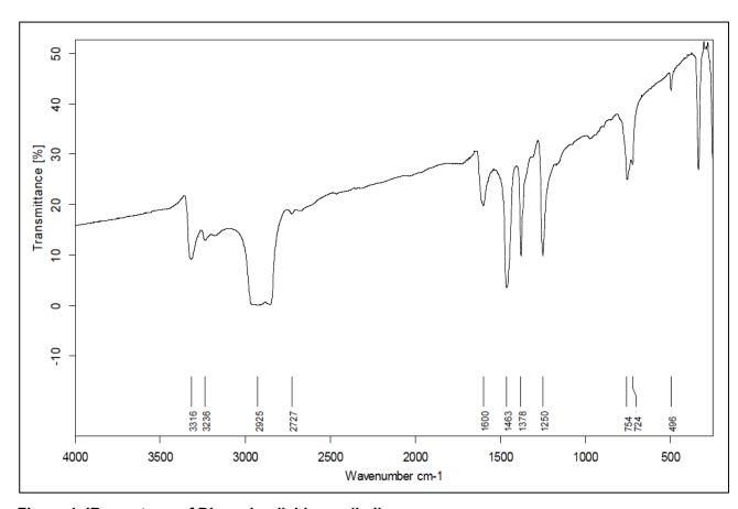
Figure 1. IR spectrum of Diamminedichloropalladium
