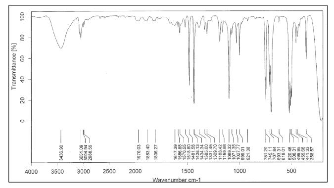
Figure 1. IR spectrum of Dichlorobis(triphenylphosphine)palladium
