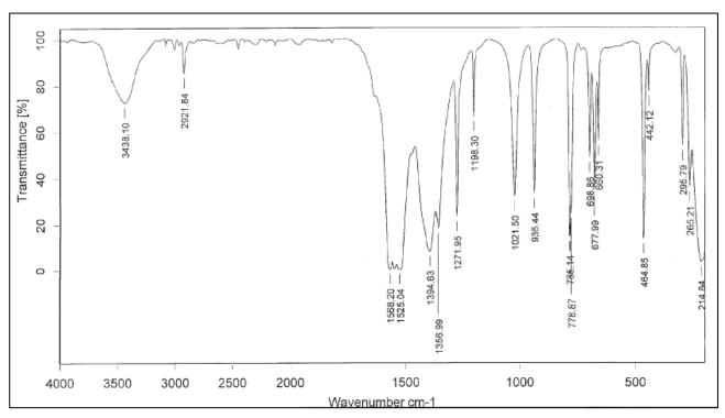
Figure 1. IR spectrum of Palladium (II) di(4-oxopent-2-en-2-oate)
