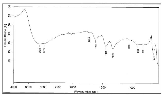
Figure 1. IR spectrum of Palladium dihydroxide
