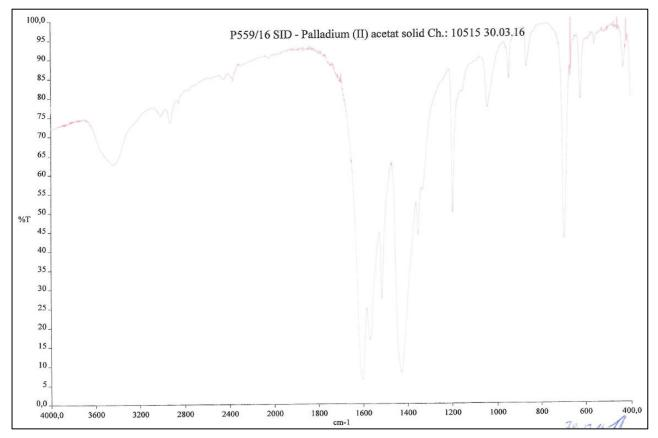
Figure 1. IR spectrum of Palladium(II) acetate
