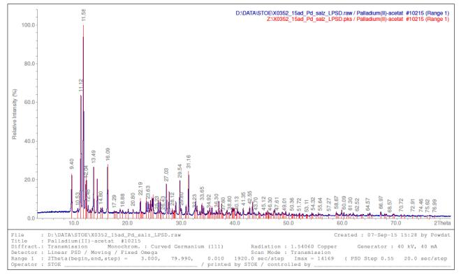
Figure 2. XRD spectrum of Palladium(II) acetate
