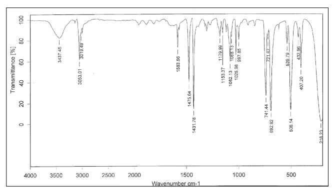
Figure 1. IR spectrum of Tetrakis(triphenylphosphine)palladium
