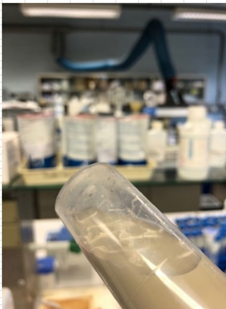
20 g \mu Ag powder in 50 ml ultrapure water after final vortex treatment.
