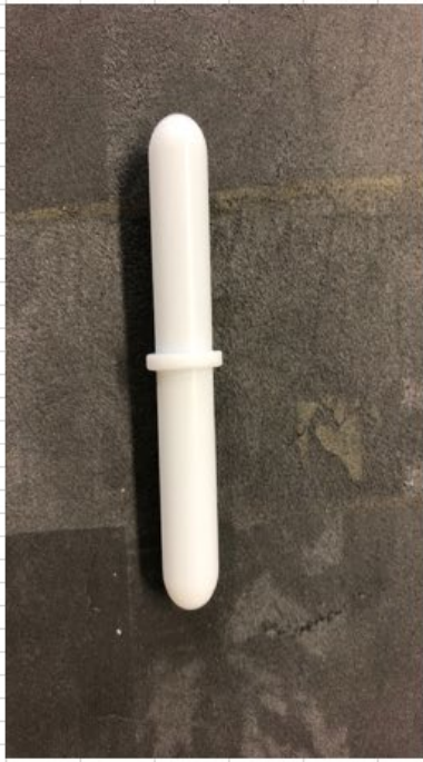
Cylindrical stirring bar with removable ring 75X12 mm VWR
