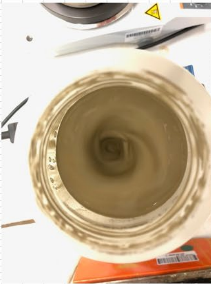
1:1:MC 400 cp 50 mg/ml Aq Bzurponian after 1hour on the tube roller and 5 minutes stirring at 900 rpm.
