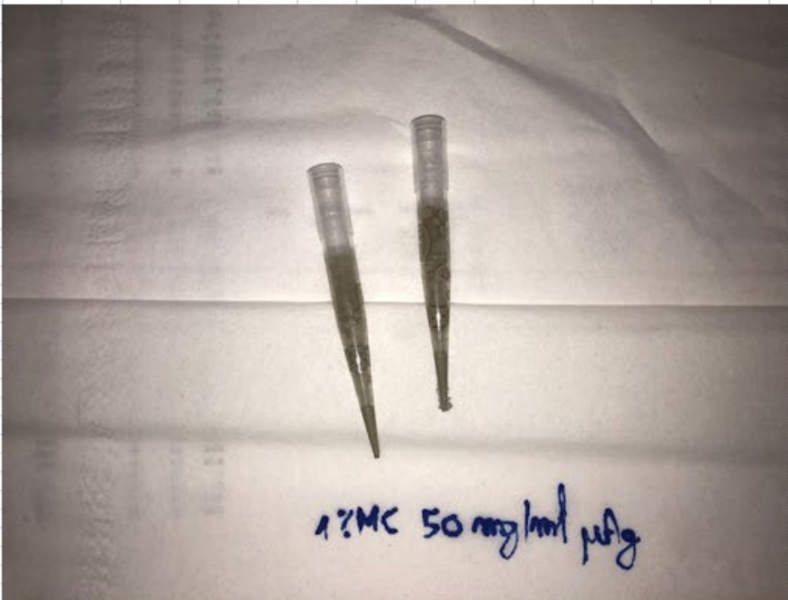
Inside of the pipette tip after taking subsample 1ml 1% MC 400cp 50 mg/ml \mu Ag suspension
