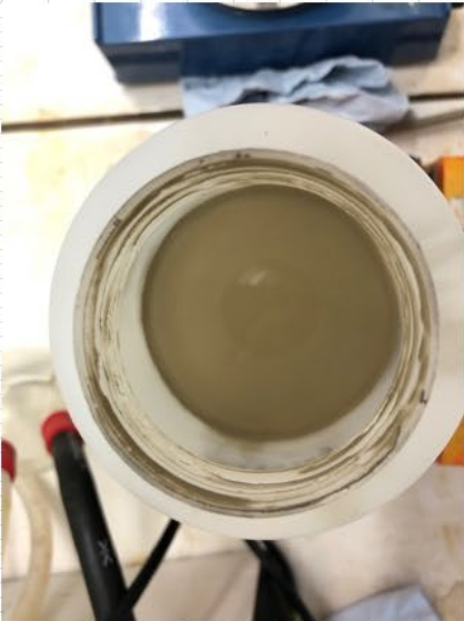
1:1 MC 400 cp 50 mg/ml Ag suspension after 20 hours in the fridge.
