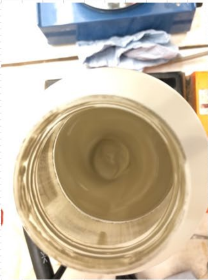
1:1:MC 400 cp 50 mg/ml Aq Azurponian after 1hour on the tube roller and 5 minutes stirring at 900 rpm.
