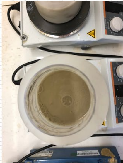
0.1:1 MC 400 cp 50 mg/ml Ag suspension after 20 hours in the fridge.
