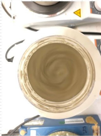
0.1:1:MC 400 cp 50 mg/ml Aq Azurponian after 1hour on the tube roller and 5 minutes stirring at 400 rpm.
