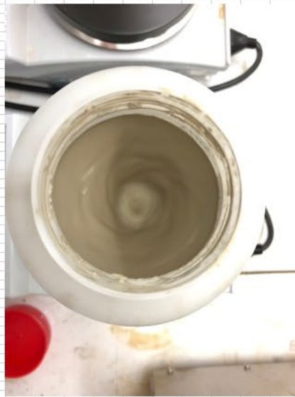
0.1:1:MC 400 cp 50 mg/ml Aq Bzurponian after 1hour on the tube roller and 5 minutes stirring at 400 rpm.
